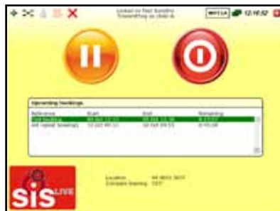
8 uPod auto transmits at the booked time and stops when the transmission is complete
